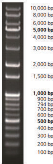
5.0 \mu l loading / 5 mm lane width 1.0% TAE agarose gel with stained EtBr
